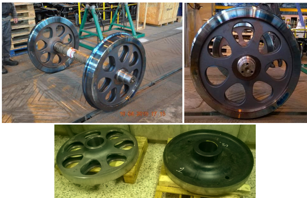
Fig. 14 Top: the very first wheelset with Liberty Wheels (16.04.2019). Bottom: comparison of the Liberty Wheel with the original wheel centre
