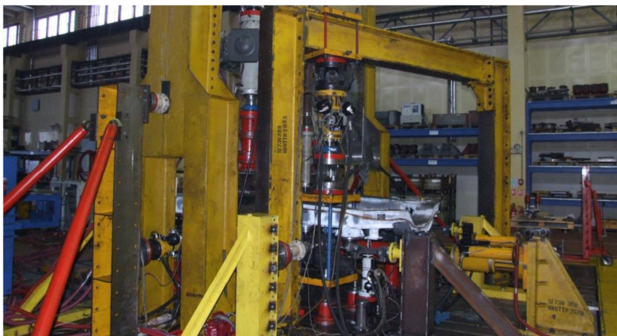
Fig. 8 Bogie frame of the locomotive class 744.1 mounted in the testing bench.
