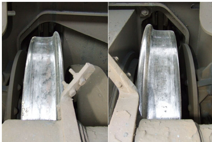
Fig. 1 Asymmetric profile wear (picture of left and right wheel of one wheelset)
