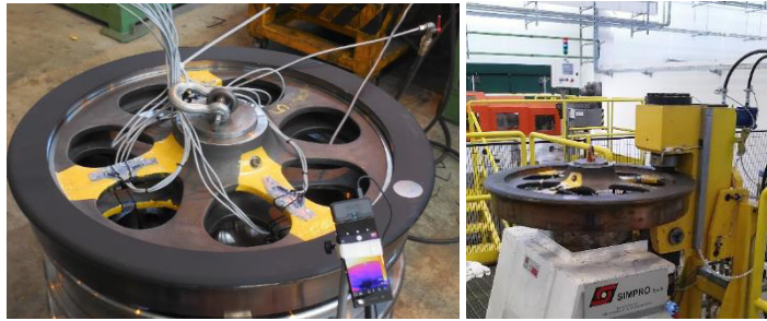
Fig. 15 Measuring the strains in the spokes by means of ER strain gauges during cooling of the tyre (left). The Liberty Wheel under test mounted in the full-scale facility (right).
