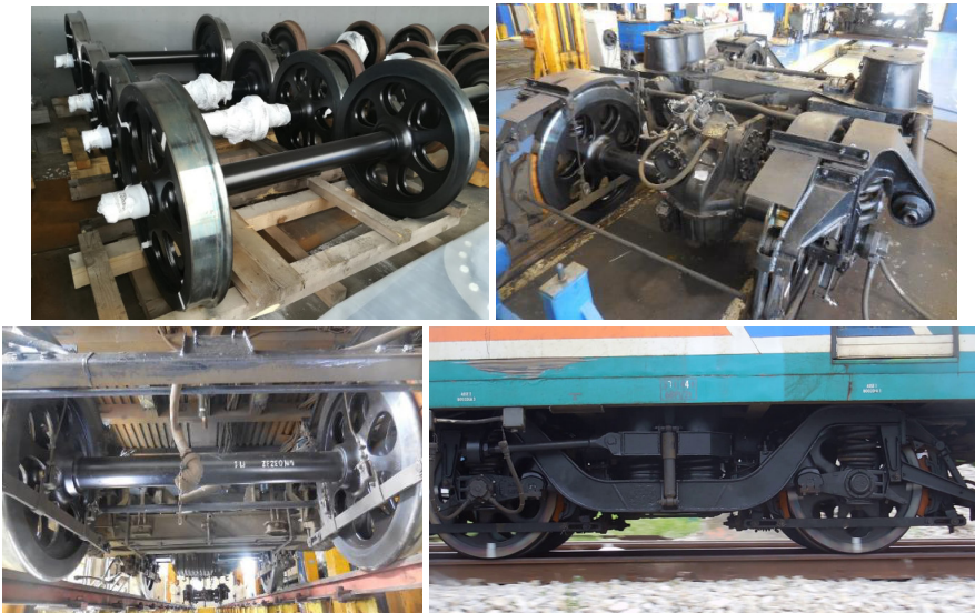
Fig. 16 Liberty wheels tested on the DMU vehicle ALn668.1053 (14.05.2019, Iseo, Brescia, Italy).
