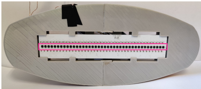
Fig. 3 Magnetic field with rectangular profile and varying air gap
