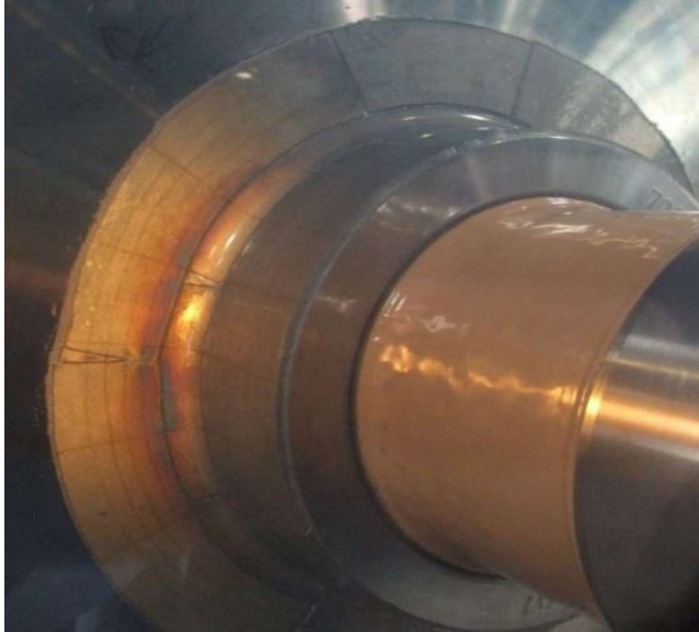
Fig. 8. The fringe distribution of inner surface B/I in crossed polarisation state of pressed wheel “B”
