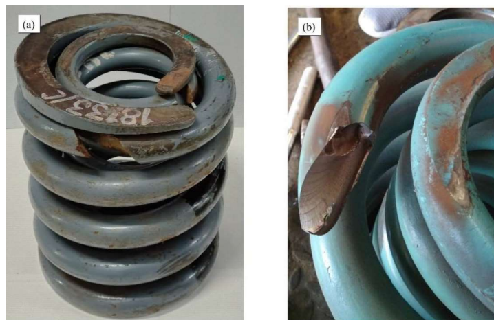
Figure 1 (a) Broken inner and outer spring of primary suspension, (b) Exploded view of outer spring failure
