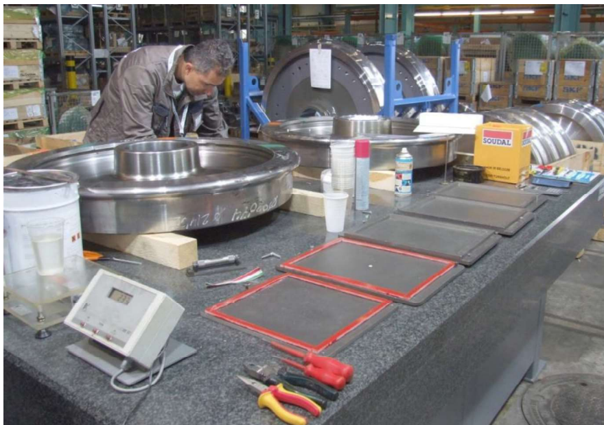
Fig. 6. Railway wheels under test on the assembly table
