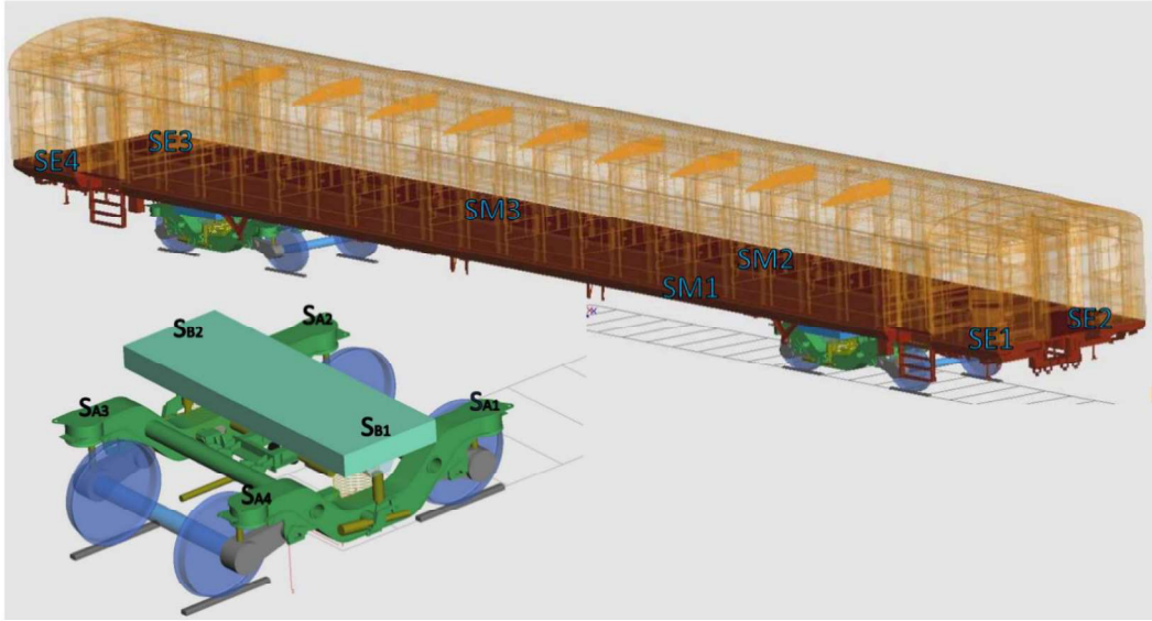
Figure 2 Simpack MBD model and sensors locations
