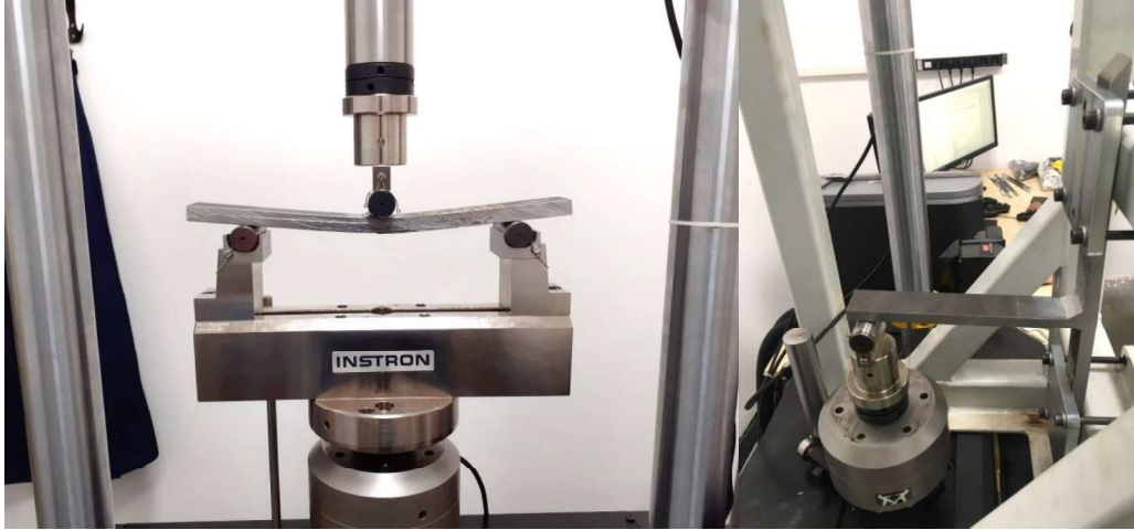
Fig 6. Fatigue testing setup for butt welded (left) and fillet welded (right) samples
