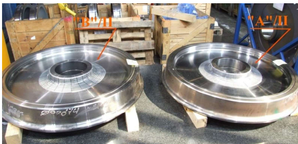
Fig. 7. The wheel-pair prepared for investigation with coating and network
