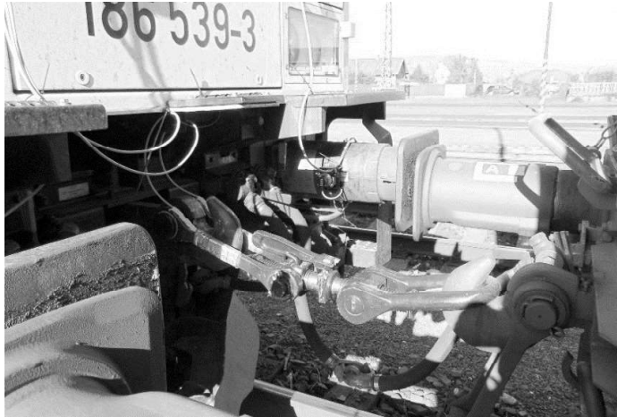
Fig. 6 Instrumented screw coupling on the locomotive
